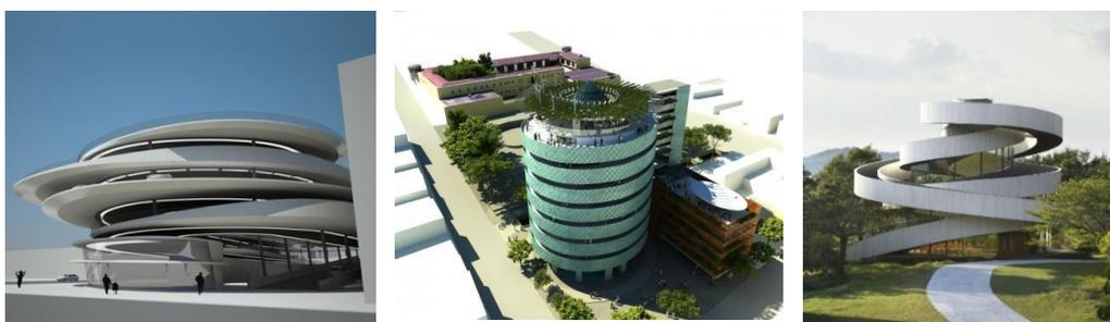
Figure 2. Examples for ruled helicoidal shells
