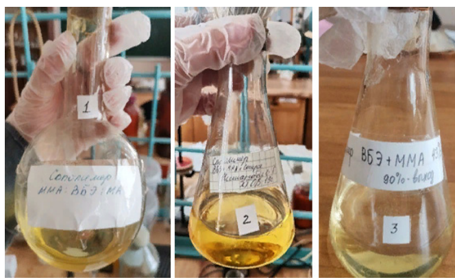
Figure 3. Finished copolymer materials for coating application Source: photo by I. Volokitina
