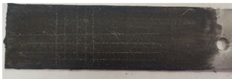
Figure 20. Example of scratch grid application Source: made by V. Merkulov
