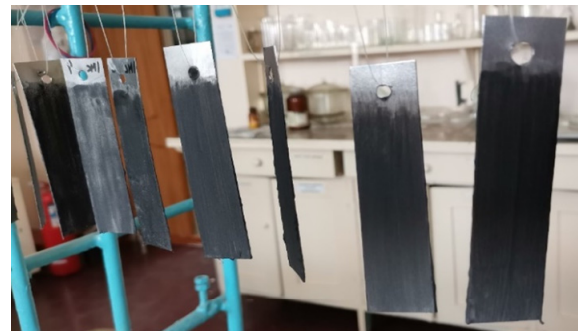
Figure 6. Polymer coating with microsilica filler Source: photo by A. Yepaneshnikova
