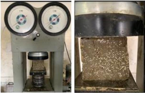
**Figure 1.** Testing for compressive strength
