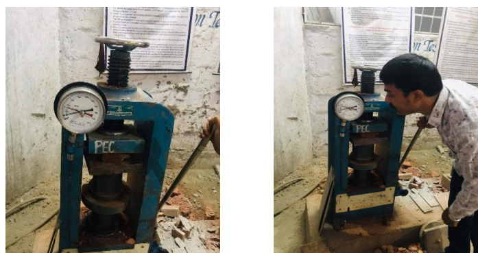
Figure 4. Testing of brick samples in lab
