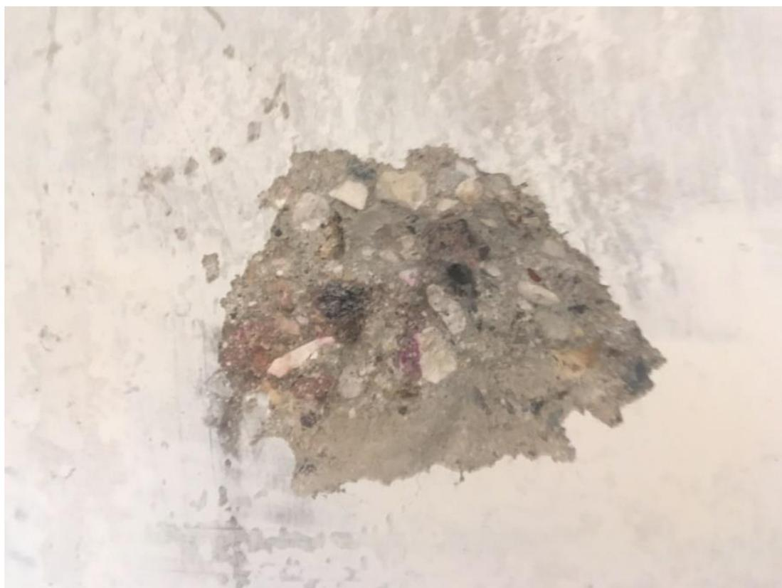
**Figure 3.** Absence of visible signs of concrete carbonization from the results of phenolphthalein test
