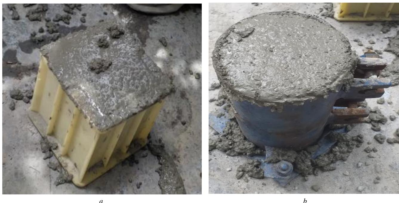
Figure 5. Cube (a) and cylinder (b) samples
