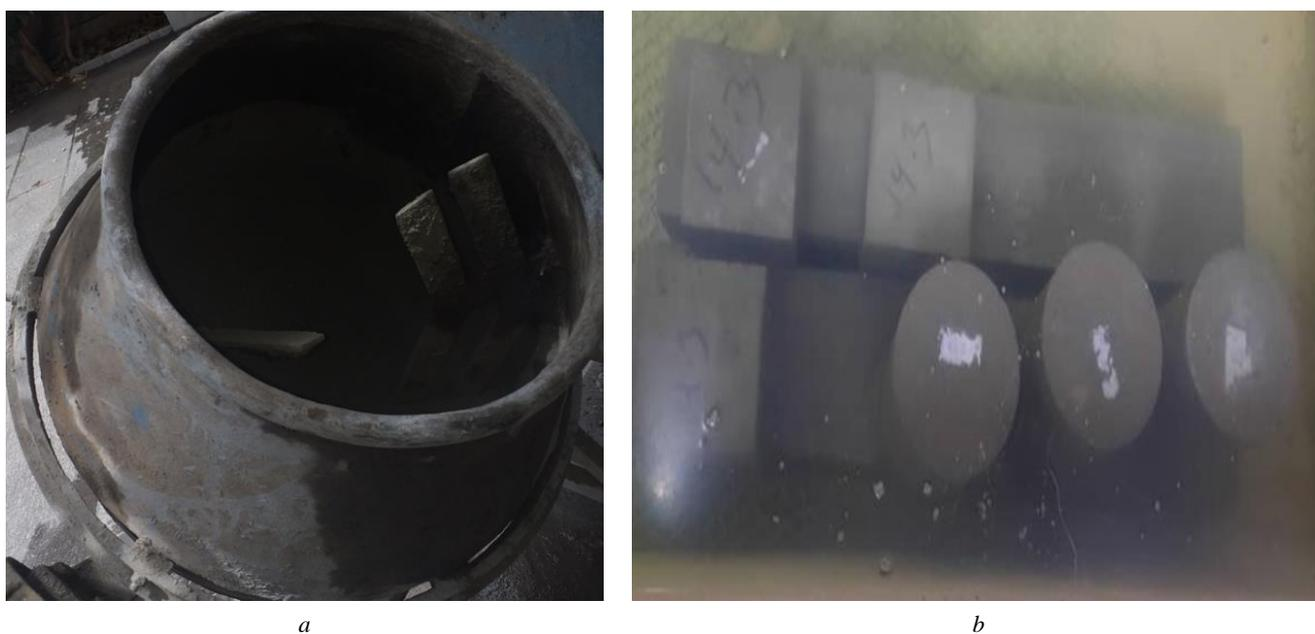
**Figure 6.** The pan mixture of laboratory (a) and molded concrete samples under water (b)
