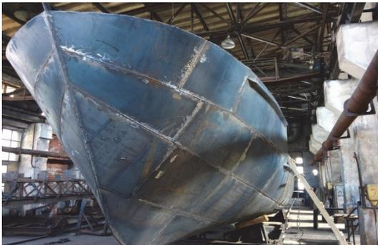
**Figure 1.** The erection of steel ship hull
