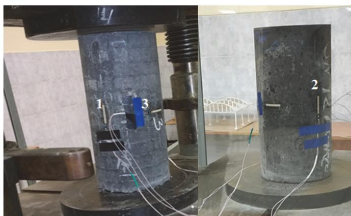
**Figure 5.** Strain gauge sensor location on ECC cylindrical column
