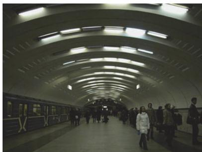
**Figure 4.** Babushkinskaya metro station, Moscow, Russia, 1978. The illumination of the station is provided by lamps, which are located in the slots of the elliptical arch
