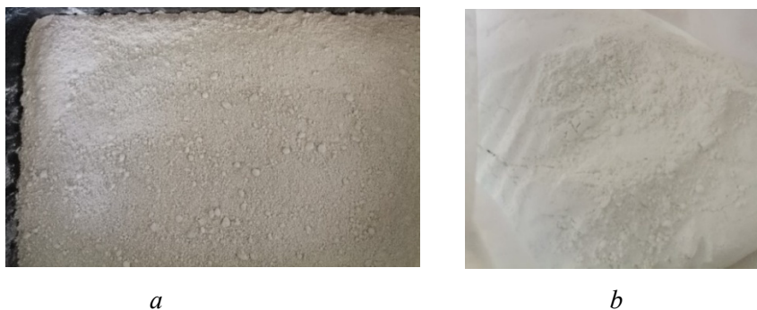
Figure 1. Filler appearance: a — microsilica; b — titanium oxides Source: made by I. Volokitina
