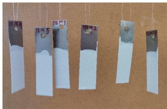
Figure 7. Combined polymer coating Source: photo by A. Yepaneshnikova
