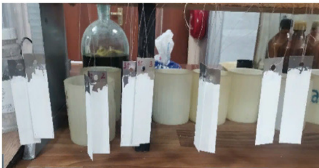
Figure 5. Polymer coating with titanium oxide filler Source: photo by A. Yepaneshnikova
