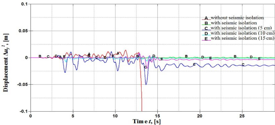
**Figure 8.** Displacement of the top of the 1st floor of the 9-storey building relative to its bottom along the  $Y$  axis
