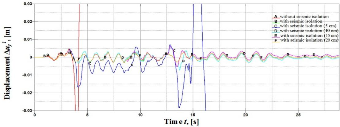
**Figure 10.** Displacement of the top of the 1st floor of the 16-storey building relative to its bottom along the  $X$  axis
