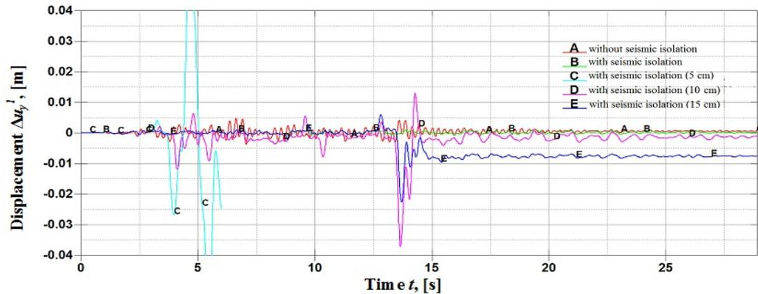
**Figure 6.** Displacement of the top of the 1st floor of the 5-storey building relative to its bottom along the  $Y$  axis
