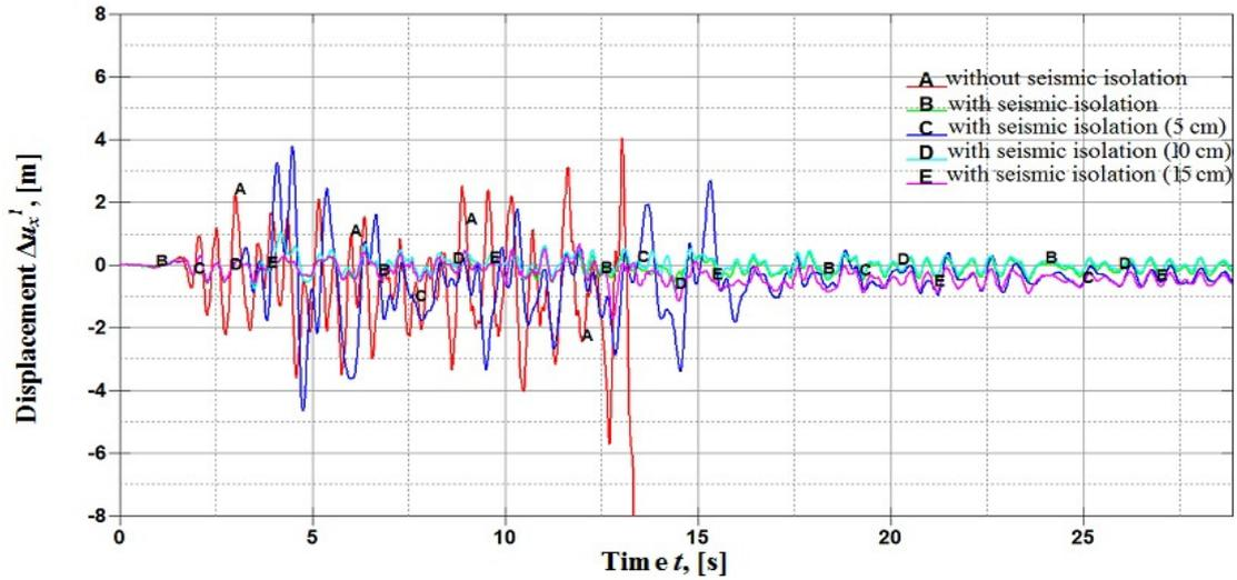
**Figure 7.** Displacement of the top of the 1st floor of the 9-storey building relative to its bottom along the  $X$  axis
