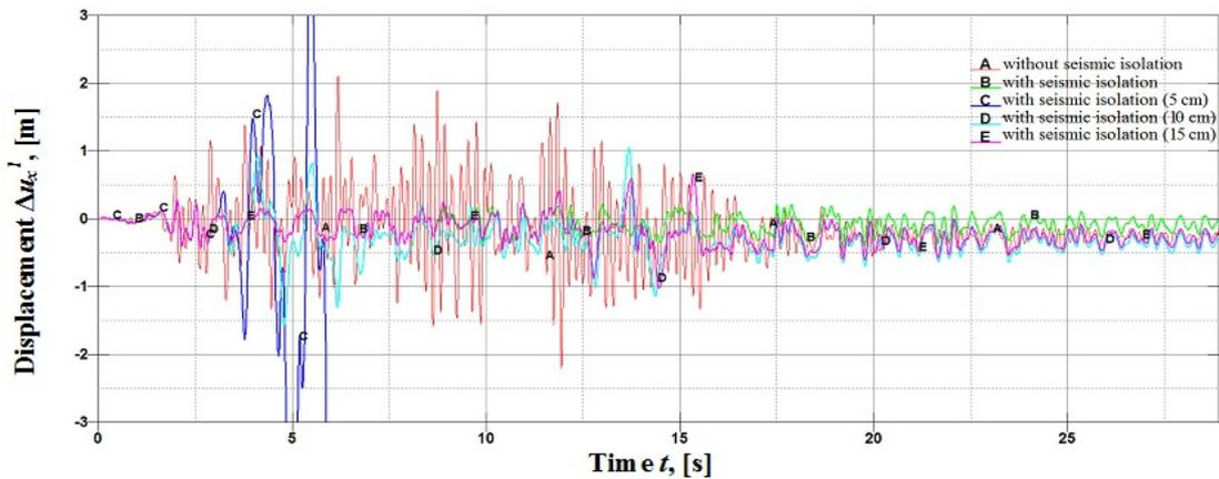
**Figure 5.** Displacement of the top of the 1st floor of the 5-storey building relative to its bottom along the  $X$  axis
