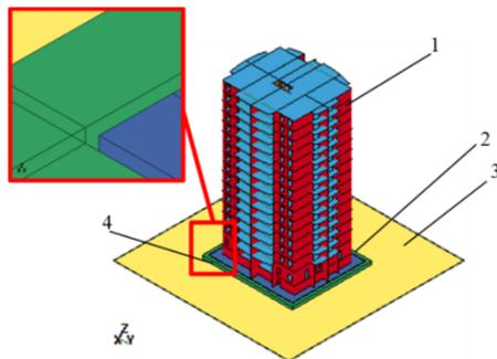
**Figure 1.** Model of a 16-storey building with a sliding belt and an elastic limiter of horizontal displacements:
