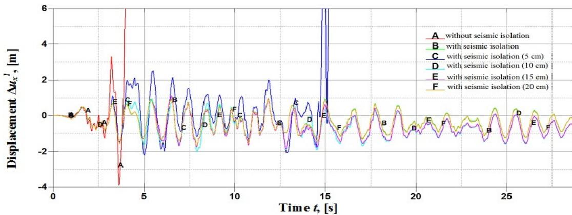
**Figure 9.** Displacement of the top of the 1st floor of the 16-storey building relative to its bottom along the  $X$  axis
