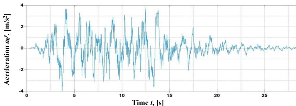
**Figure 4.** Single-component earthquake accelerogram in Y direction for the 16-storey building
