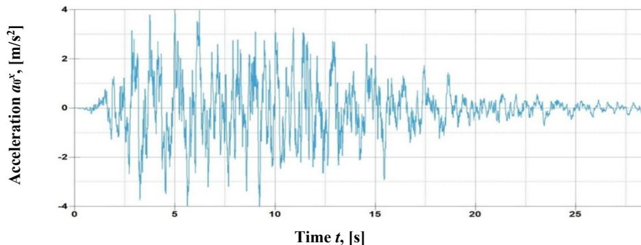
**Figure 3.** Single-component earthquake accelerogram in X direction for the 16-storey building
