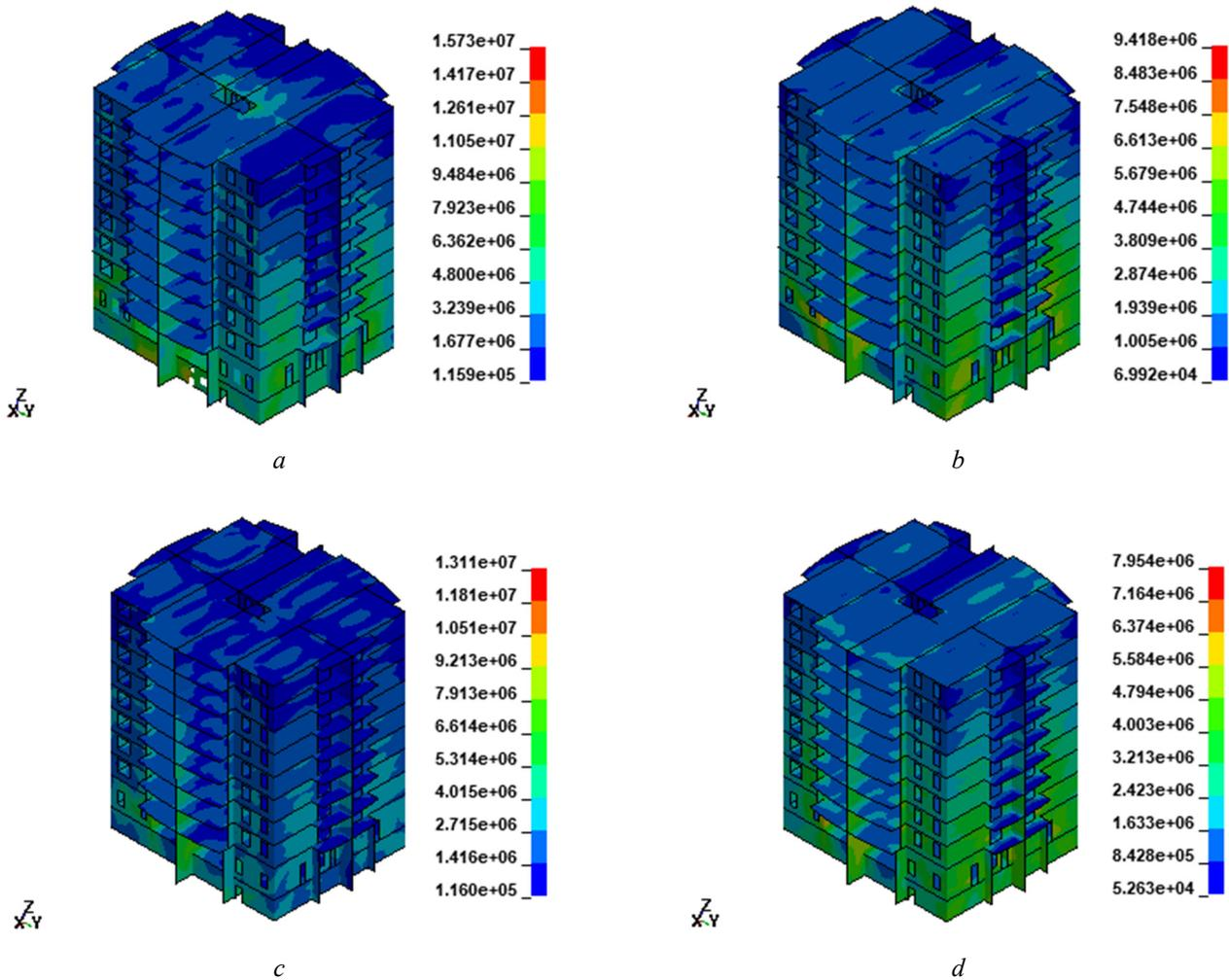
**Figure 11.** Stress intensity distribution (in units of Pa) at time  $t=13.20$  s of the 9-storey building with seismic isolation and elastic limiter of horizontal displacements at a distance of:  $a$  — 5 cm;  $b$  — 10 cm;  $c$  — 15 cm;  $d$  — 20 cm
