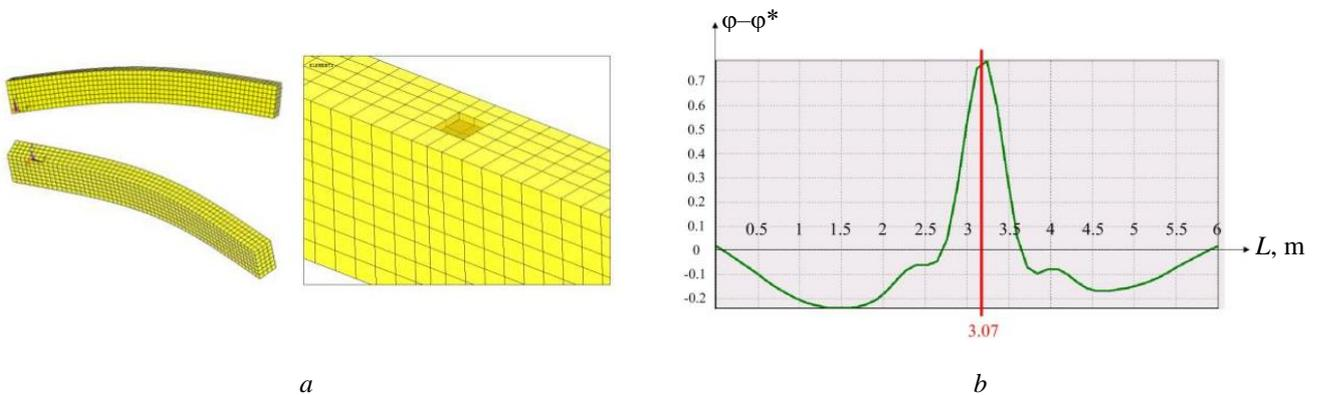
**Figure 1.** Defect detection by modal convergence method:
