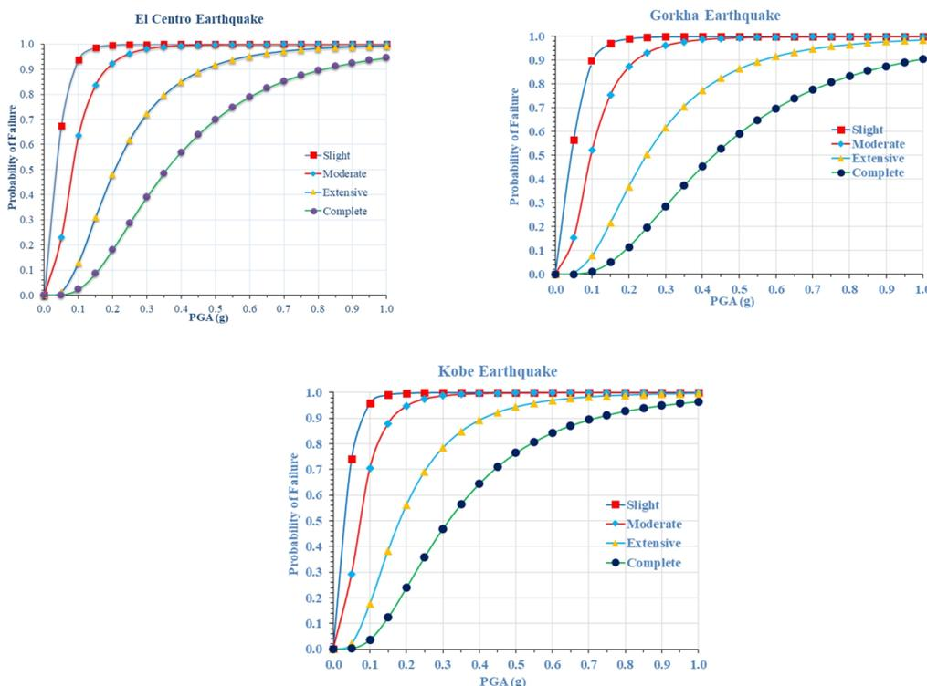
**Figure 9.** Fragility Curve of Old Newari Building for various Damage States at El Centro Earthquake
