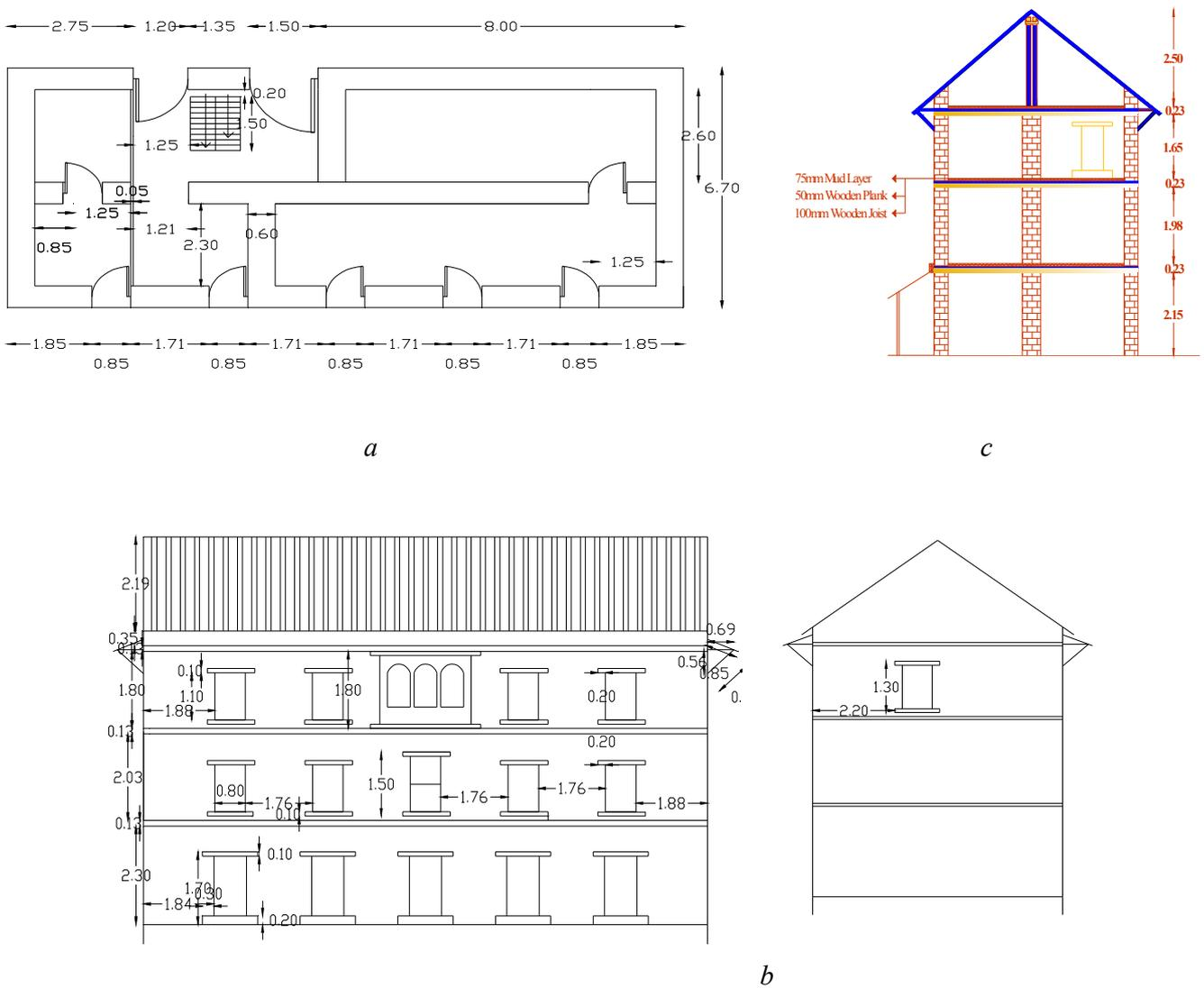
**Figure 3.** Details of studied building structure:
