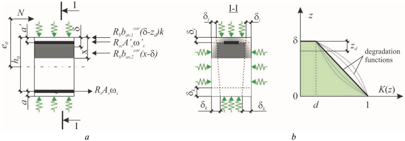
**Figure 1.** Design scheme of an eccentrically compressed corrosion-damaged reinforced concrete element: a – cross-sectional design scheme; b – a general view of the degradation function for the concrete layer damaged with corrosion
