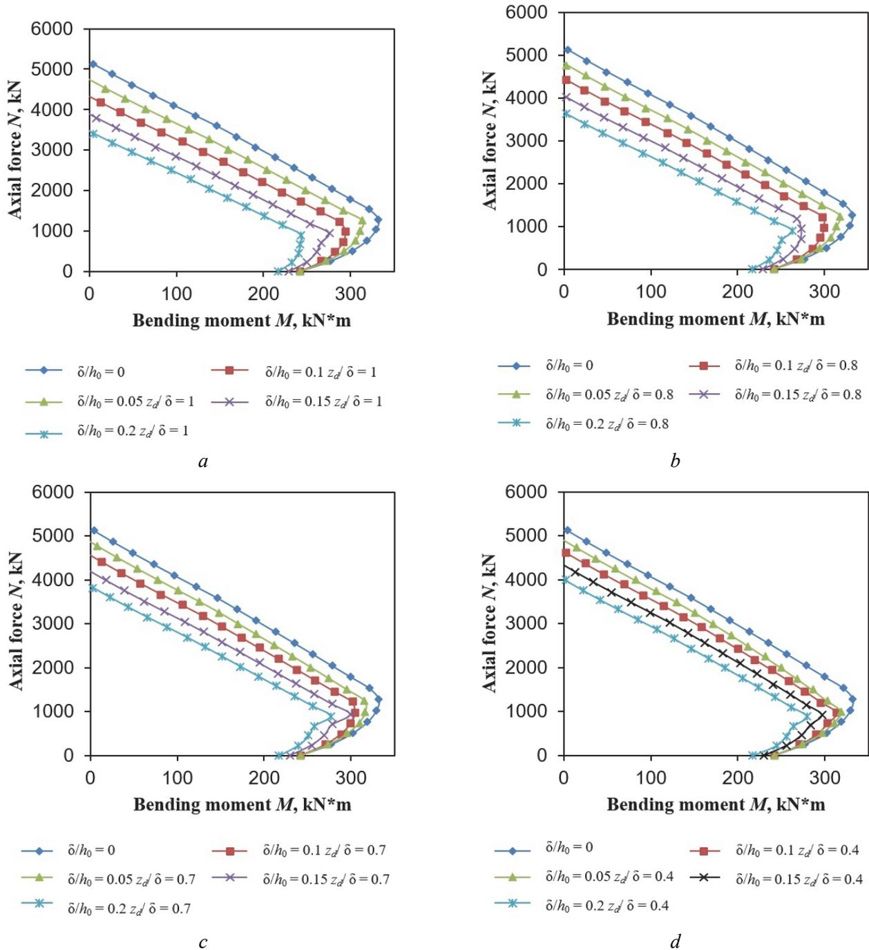
**Figure 2.**  $M - N$  interaction diagrams for corrosion-damaged eccentrically compressed reinforced concrete elements with slenderness ratio  $\lambda_{ti} = 8$  depending on the relative depth of corrosion damage:
