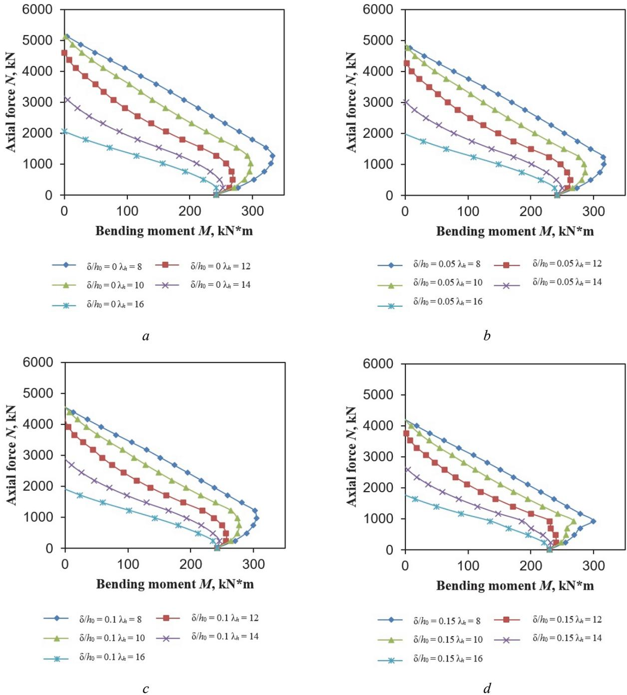
**Figure 3.**  $M - N$  interaction diagrams depending on the slenderness ratio  $\lambda_h$  of eccentrically compressed reinforced concrete elements for  $z_d/\delta = 0.6$ :
