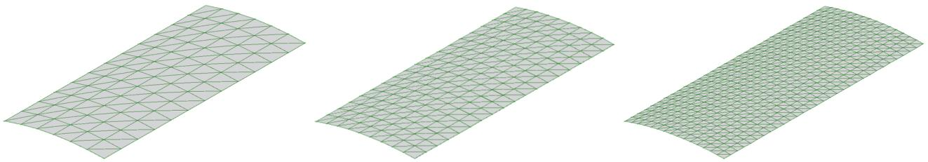
**Figure 18.** Finite element models for calculating a laminated panel
