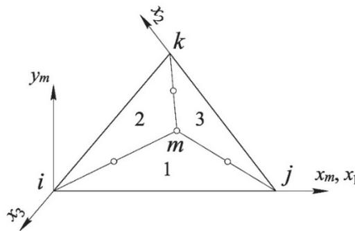
**Figure 3.** R.W. Clough & J.L. Tocher triangular finite element formation
