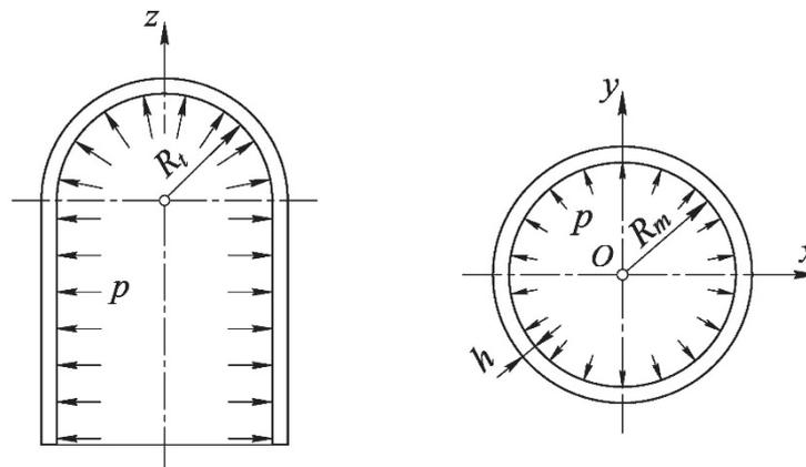
Figure 14. To the calculation of a tank
