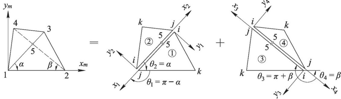
Figure 4. Forming a quadrangular finite element
