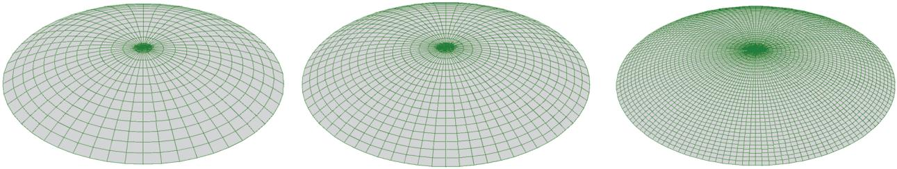
Figure 10. Finite element models of a spherical shell
