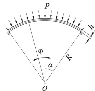
**Figure 9.** To the calculation of a spherical shell
