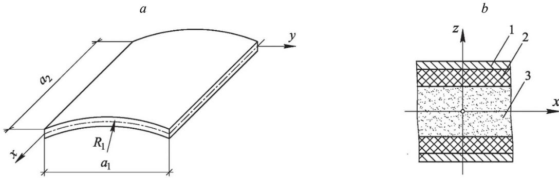
**Figure 17.** To the calculation of a laminated cylindrical panel:
