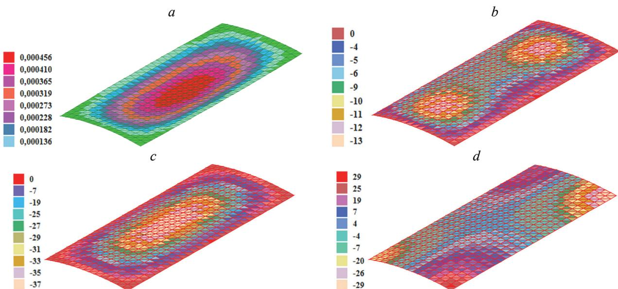
**Figure 19.** Calculating results of a laminated cylindrical panel:
