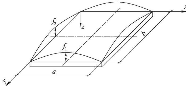
Figure 5. To the calculation of a shallow shell
