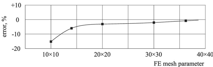
**Figure 8.** Convergence graph of calculation results for displacements
