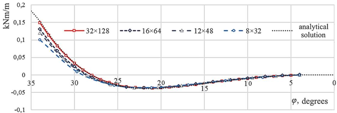
Figure 12. Convergence graph of the calculation results by the meridional bending moments  $M_x$
