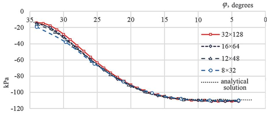
Figure 13. Convergence graph of calculation results for circumferential stresses  $\sigma_\varphi$ .
