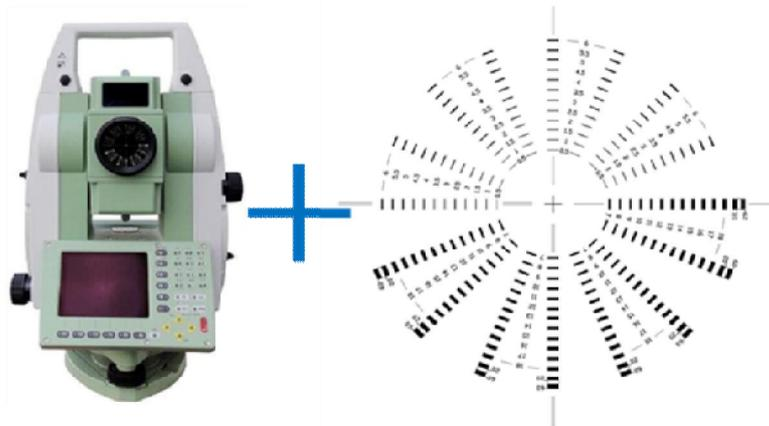
Fig. 2. The main unit of a total station and a built-in crack scale
