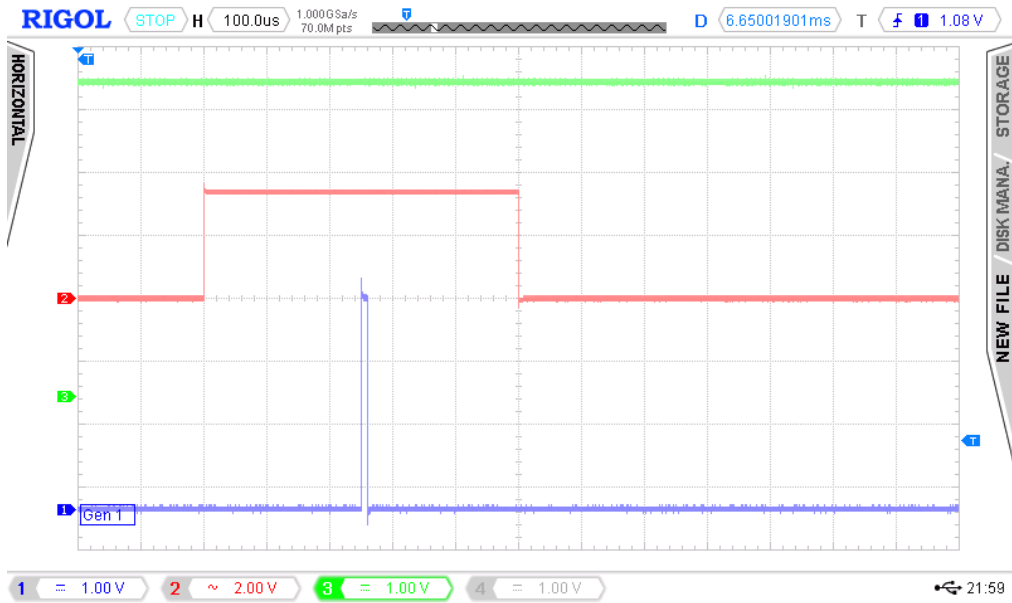
(b) the 3-rd pulse of the pulse train with advances of 250 microseconds
