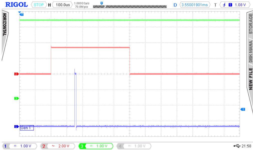
(a) the 2-nd pulse of the pulse train with advances of 150 microseconds
