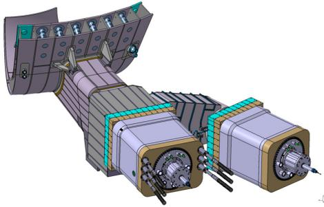
Figure 2. Vacuum vessel cryoport with installed torus cryopump. CATIA drawing
