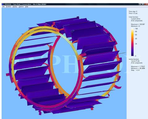
Figure 18. Steady state distribution of eddy current over the 4K panels assembly of the cryopump caused by simultaneous discharge of CS and all PF coils. The step of current lines is 0.5A
