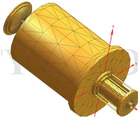
Figure 5. Calculation model of cryopump assembly
