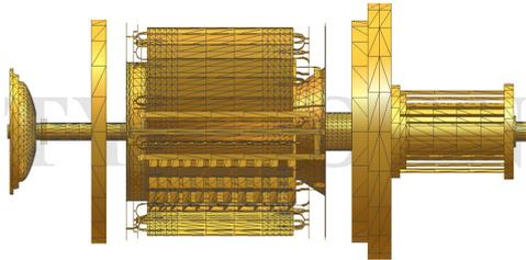
Figure 14. Calculation model of torus cryopump. The carrier tube of housing and carrier tubes of 80K radiation shield are not shown
