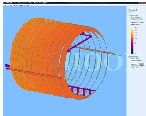
Figure 17. Steady state distribution of eddy current over the 80K louvers assembly of the cryopump caused by simultaneous discharge of CS and all PF coils. The step of current lines is 0.2A
