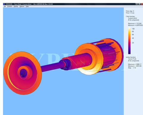
Figure 19. Steady state distribution of eddy current over the valve assembly of the cryopump caused by simultaneous discharge of CS and all PF coils. The step of current lines is 10A
