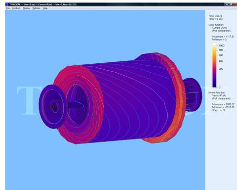
Figure 15. Steady state distribution of eddy current over the cryopump assembly caused by simultaneous discharge of CS and all PF coils. The step of current lines is 10A
