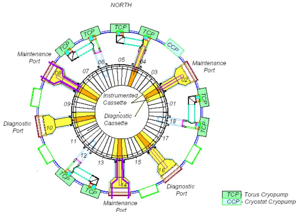
Figure 1. Arrangement of 8 Torus Cryopumps (TCP) in the ITER machine
