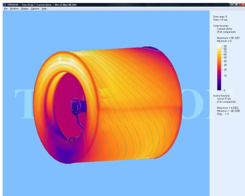
Figure 16. Steady state distribution of eddy current over the 80K assembly of the cryopump caused by simultaneous discharge of CS and all PF coils. The step of current lines is 5A
