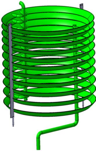
Figure 8. Torus cryopump 80K louvers assembly. CATIA drawing.
