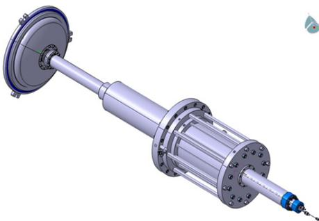
Figure 12. Torus cryopump valve assembly. CATIA drawing.
