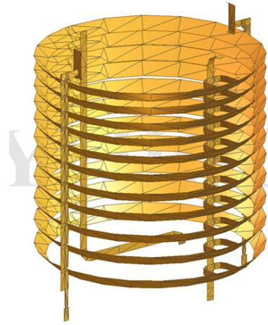
Figure 9. Calculation model of 80K louvers assembly of torus cryopump
