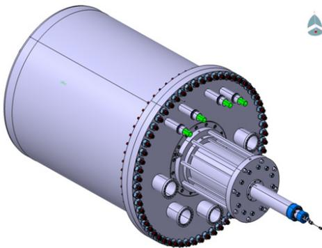
Figure 4. Cryopump assembly. CATIA drawing
