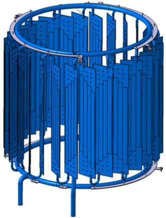
Figure 10. Torus cryopump 4K panels assembly. CATIA drawing
