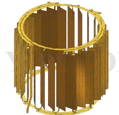
Figure 11. Calculation model of 4K panels assembly of torus cryopump
