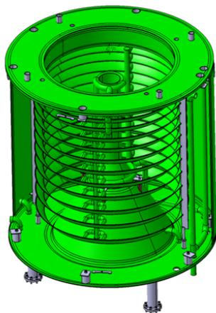
Figure 6. Torus cryopump 80K assembly. CATIA drawing
