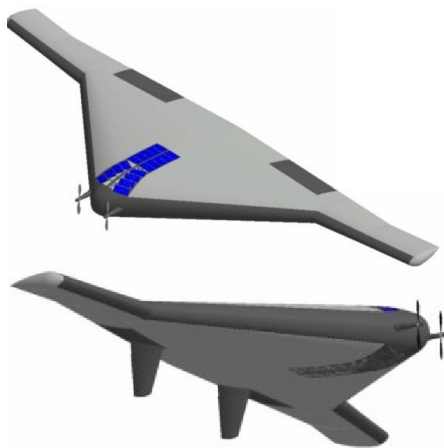
Figure 4. Venus Atmospheric Maneuverable Platform (VAMP) — Inflatable airplane Source: by G. Lee et al. [12]
