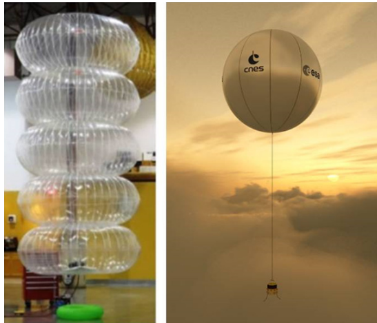
Figure 2. Balloon probe with payload of the Vega project Source: by Glaze et al. [20]
