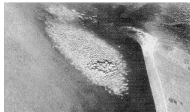
Figure 4. Hub vortex cavitation Source: Sezen S., Atlar M. [22]
