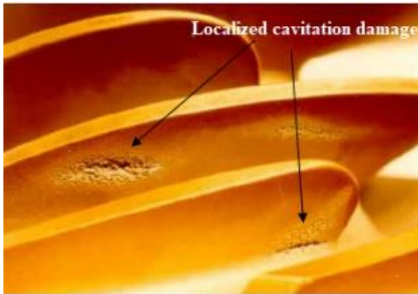
Figure 1. Localized cavitation damage and severe cavitation erosion on a pump blade Source: Brennen C.E. [18]
