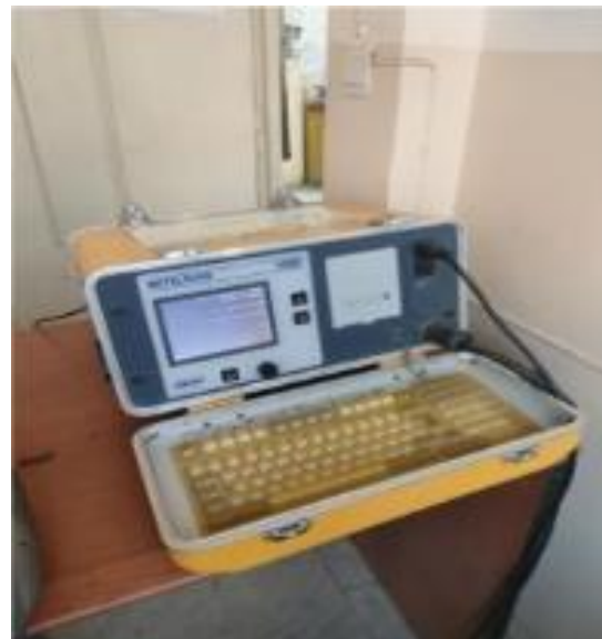
Figure 4. Metal scanning device model ARUN 1650 Source: made by the authors
