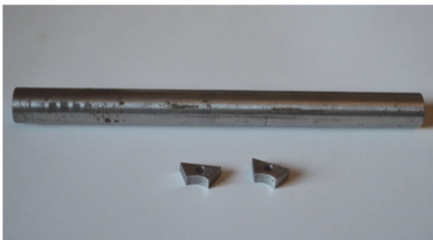
Figure 2. Sample and nozzles for measuring coercive force
