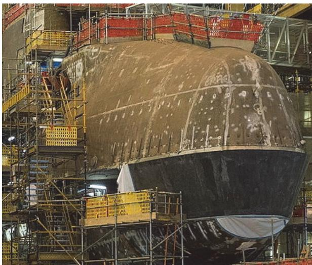
**Figure 7.** Submarine hull manufacturing using segments of developable skin (Crown Copyright 2013, by Andrew Linnett, www.defenceimages.mod.uk, photo 45155780.jpg)
