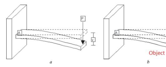
Figure 2. Deflecting cantilever beam
