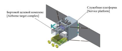
**Рис. 1.** Общий вид КА ДЗЗ [**Figure 1.** General view of the remote sensing spacecraft]
