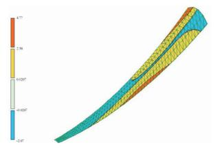
Figure 12. Fields of torques, kNm/m
