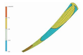
Figure 7. Fields of normal stresses in the radial direction, kN/m<sup>2</sup>
