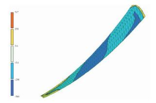
**Figure 8.** Fields of normal stresses in the circumferential direction, kN/m<sup>2</sup>
