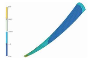
**Figure 10.** Fields of bending moments in the radial direction, kNm/m
