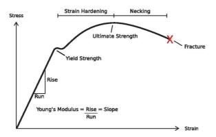
Figure 1. Material stress-strain diagram
