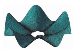
Figure 4. The finite element model of the paraboloid shell
