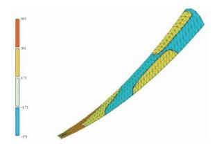
Figure 9. Fields of tangential stresses,  $kN/m^2$
