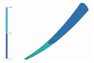
**Figure 11.** Fields of bending moments in the circumferential direction, kNm/m
