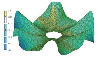
Figure 6. Fields of vertical displacements of the shell
