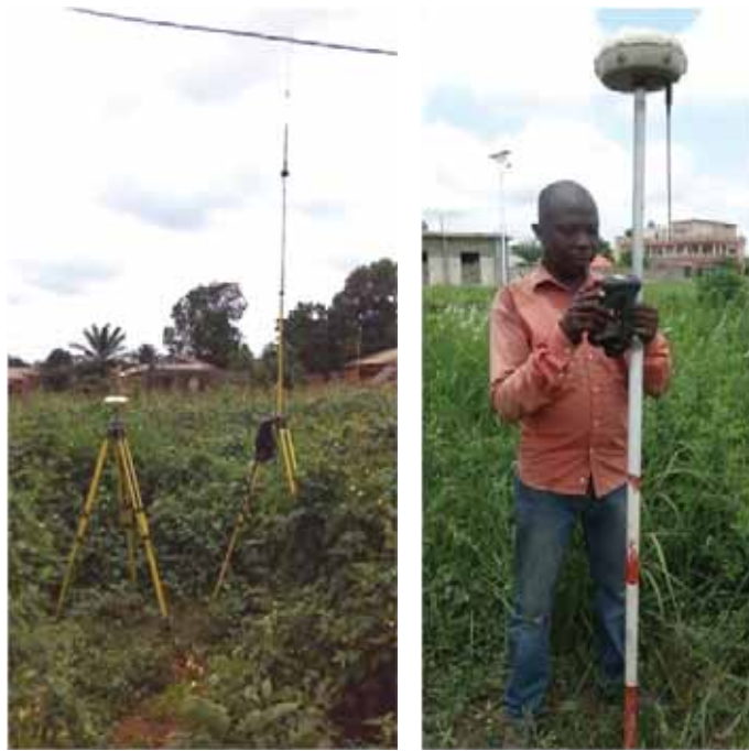
Figure 2. Base and radio as well as the mobile of the receiver GNSS CHC X 91
