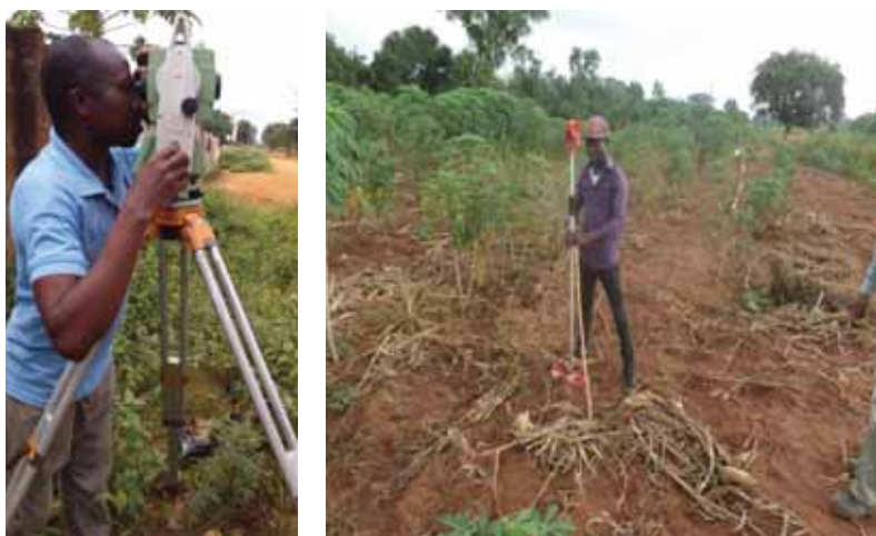
Figure 3. Surveying with the total station LEICA TS06
