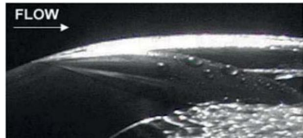
**Figure 3.** Lead edge cavitation
