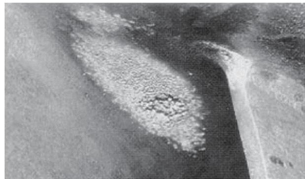
**Figure 4.** Hub vortex cavitation
