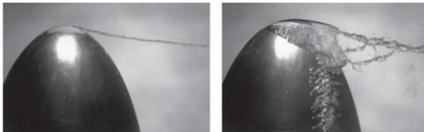
**Figure 2.** Cavitating tip vortices
