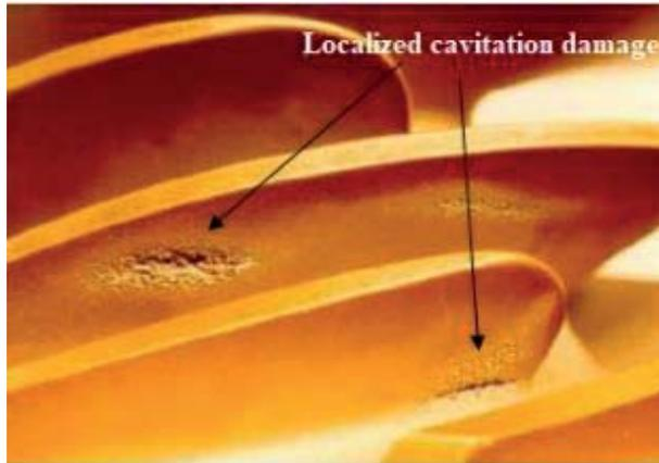
**Figure 1.** Localized cavitation damage and severe cavitation erosion on a pump blade
