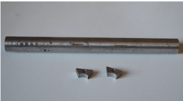
Figure 2. Sample and nozzles for measuring coercive force
