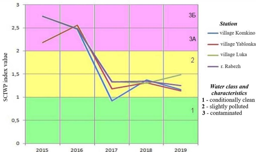
Figure 3. Values of the *SCIWP* index in the sections of the Shlinskoye reservoir for 2015–2019
