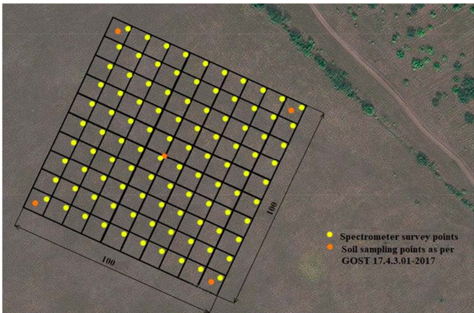
Figure 3. Survey of spectral data and soil sampling Source: compiled by the author.
