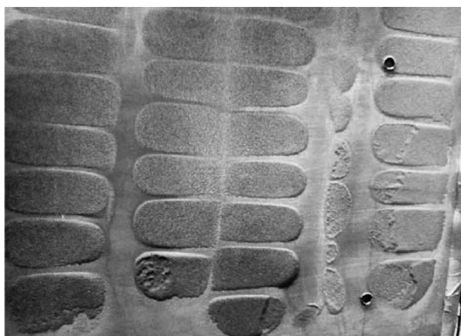
Figure 4. Photograph of the structure of precipitated dust in a laboratory electrostatic precipitator
