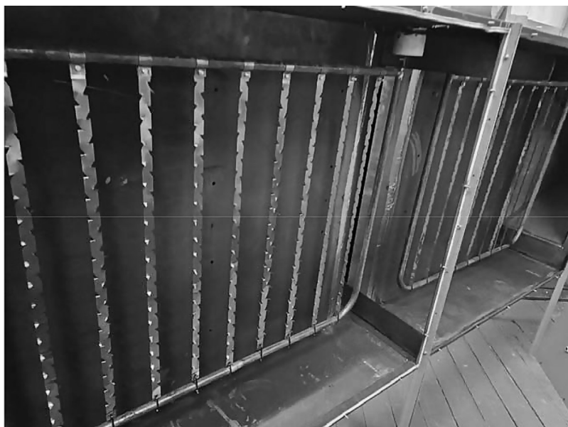
Figure 1. Laboratory electrostatic precipitator with the collecting electrode removed
