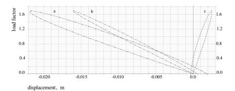
Figure 5. Variation of load factor with displacement at node 74 in the buckling zone for C2 (a) vertical displacement component (b) (c) horizontal displacement components
