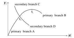
Figure 1. Load path of a structure
