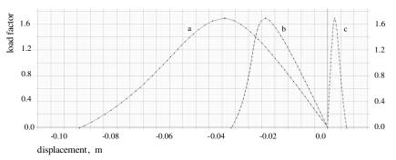
Figure 4. Variation of load factor with displacement at node 42 in the buckling zone for C2 (a) vertical displacement component (b) (c) horizontal displacement components
