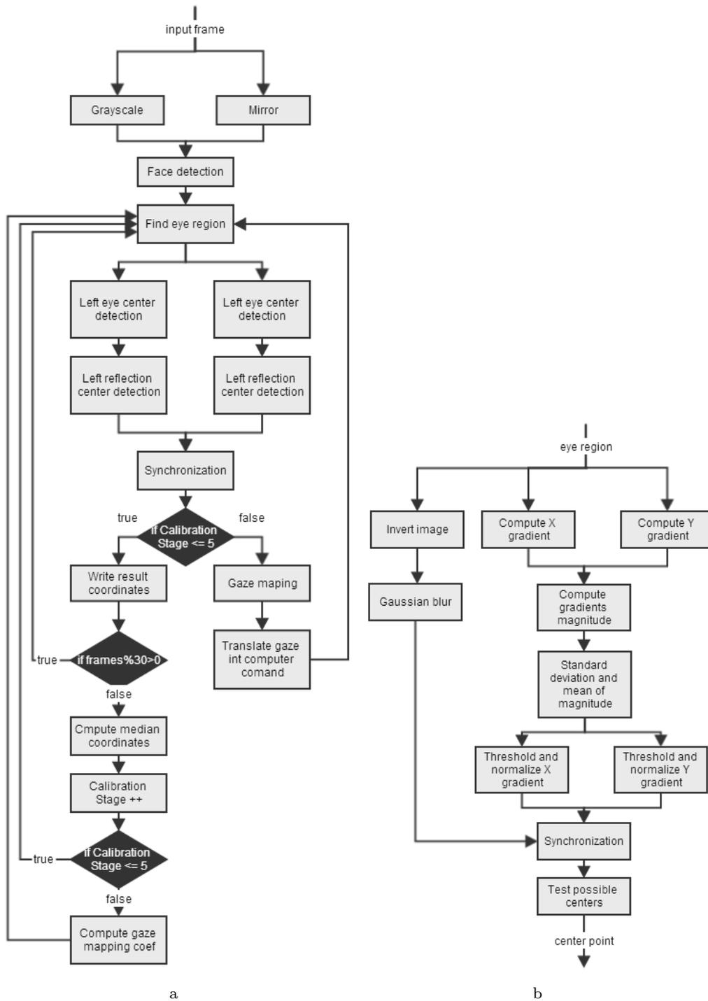
Figure 5. General algorithm flowchart (a) and Eye center localization algorithm flowchart (b)
