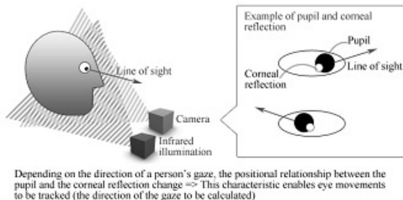
Figure 4. Graphical representation of infrared illumination approach
