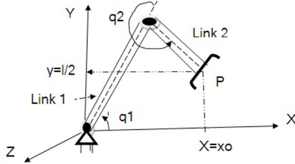
**Figure 1. Two-link manipulator**
