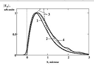
Figure 2. Electric field amplitude of the TE-mode in a single-mode waveguide with refractive index profile (2) calculated by various methods
