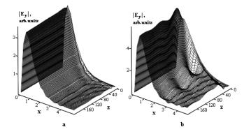
Figure 1. Field pattern in the substrate of a single-mode waveguide with exponential refractive index profile (2) computed by the BPM. The input beam width  $w = 0.47 \,\mu$ m (a),  $0.65 \,\mu$ m (b). Distances along x- and z-axes are given in micrometers
