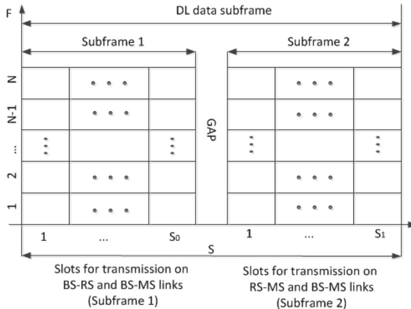
**Figure 2. Downlink data subframe for OFDMA relay-enhanced networks**
