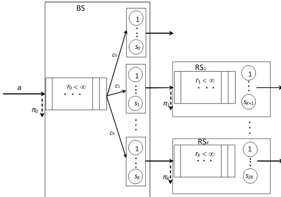
**Figure 3.** The structure of the model with overall  $S$  Chs, which are distributed between BS and RSs, and  $K + 1$  types of incoming requests
