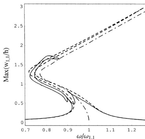
**Figure 3.** Effect of the curvature aspect ratio  $R_x/R_y$  on the shell response (maximum of the generalized coordinate  $w_{1,1}$ ) versus the excitation frequency; fundamental mode ( $m = 1, n = 1$ );  $\zeta_{1,1} = 0.004$ ; 9 dofs model; Donnell's theory
