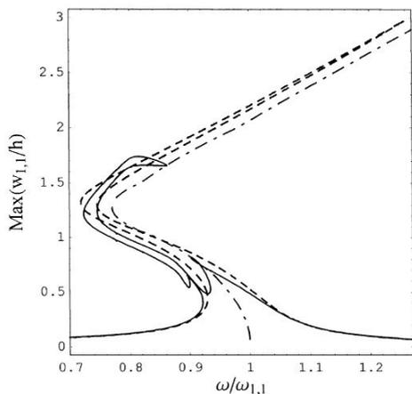
**Figure 2.** Amplitude of the response of the shell versus the excitation frequency;  $R_x/R_y = 1$  (spherical shell); fundamental mode ( $m = 1, n = 1$ ),  $\tilde{f} = 31.2$  N and  $\zeta_{1,1}\zeta_{1,1} = 0.004$ ; Donnell's theory: solid line — 22 dofs model; dashed line — 9 dofs model; dot-dashed line — backbone curve from Kobayashi and Leissa [8]
