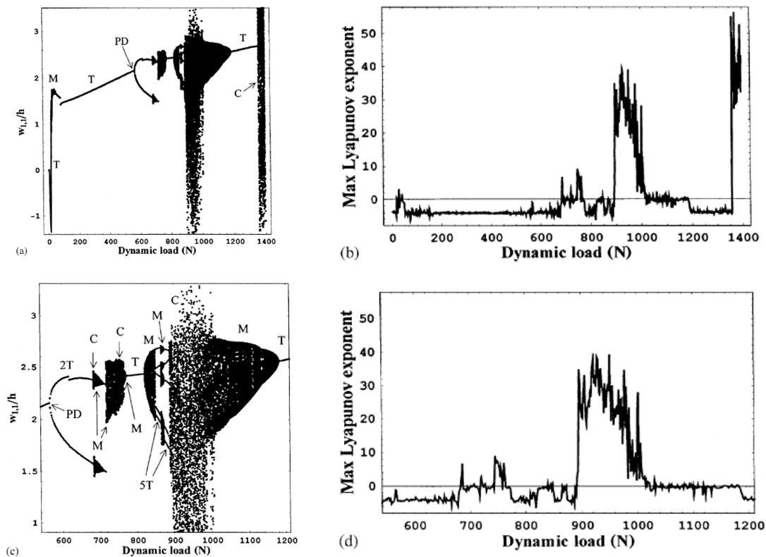
**Figure 5. Bifurcation diagram of Poincaré maps and maximum Lyapunov exponent for the spherical shallow shell under decreasing harmonic load with frequency  $\omega = 0.8\omega_{1,1}$ ;  $\zeta_{1,1} = 0.004$ ;**
